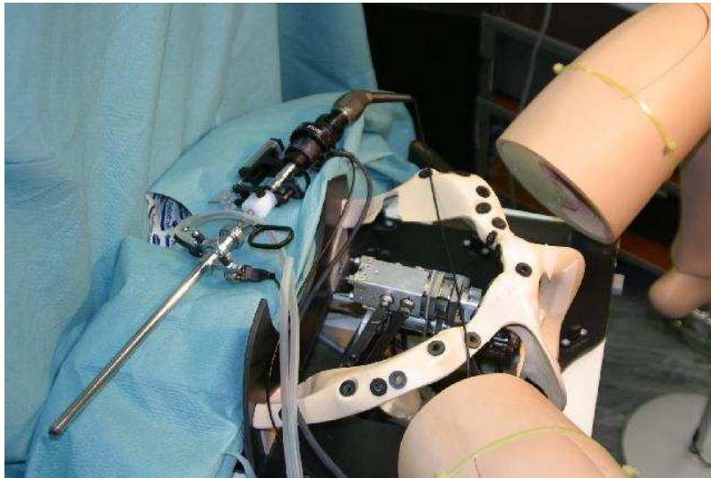
Figure 2. Haptic mechanism inside dummy.
