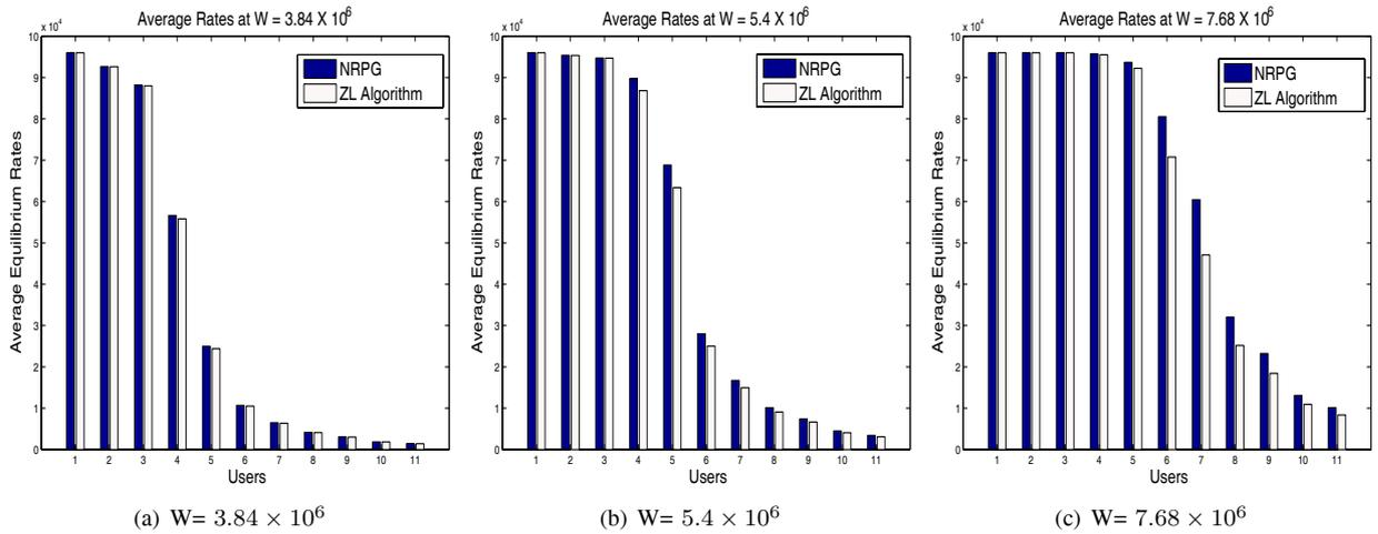
Fig. 6. The average rates yielded by the ZL algorithm and NRPG for a Monte Carlo simulation of 100 runs. User 1 is the closest to the base station and user 11 is the farthest.
