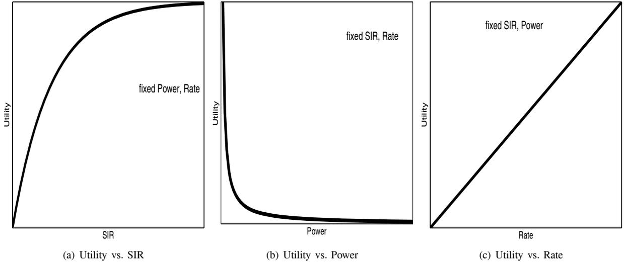
Fig. 1. The behavior of utility functions for increasing SIR with fixed power and rate, increasing power with fixed SIR and rate, increasing rate with fixed power and SIR.
