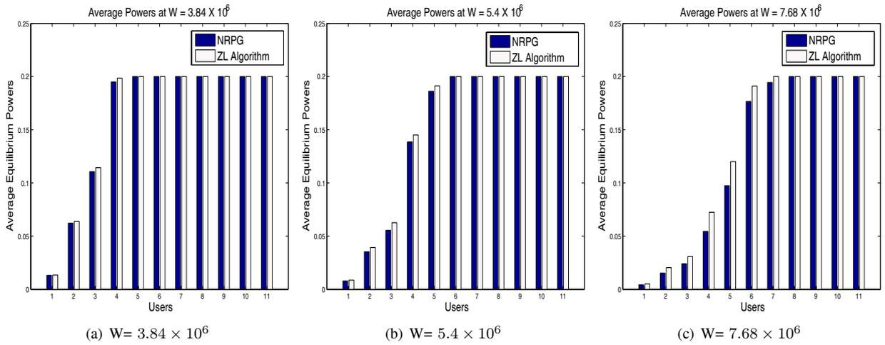
Fig. 5. The average powers yielded by the ZL algorithm and NRPG for a Monte Carlo simulation of 100 runs. User 1 is the closest to the base station and user 11 is the farthest.
